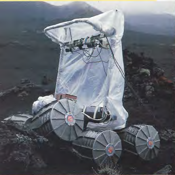
Above: The rover's camera "eyes" are on top, so the Russians had to make a visor to protect its vision, and a raincoat to cover the control and navigation equipment. Photo: George Powell
